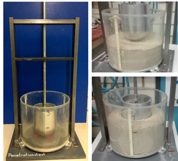
Fig. 3: New developed Penetration Test
